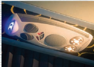
Modern design overhead console controller for Sound, Lighting and Air condition management.
