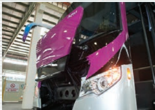
Front upward opening panel for routine maintenance checks
