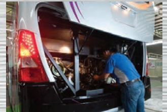
Large rear upward opening panel for easy service maintenance.
